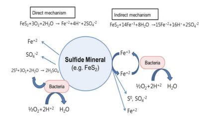
Fig. 1. Bacterial mechanism for metal sulfide dissolution. In the direct mechanism, bacteria attach directly to the sulfide mineral surface and, with aid of  $O_2$  and  $CO_2$ , bacteria dissolve metal ions to the solution phase and sulfide is changed to sulfate. In the indirect mechanism, bacteria take up  $O_2$  and  $CO_2$  and oxidize Fe<sup>+2</sup> (energy source) to Fe<sup>+3</sup>, which dissolve metal ions. After releasing metal ion, Fe<sup>+3</sup> is again reduced to Fe<sup>+2</sup>.
